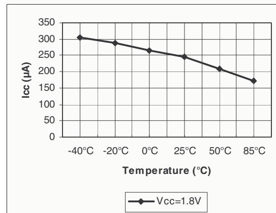
**Figure 6.** Icc vs. temp. Isink=2mA
