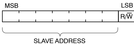
Figure 31. First Byte after START Procedure
