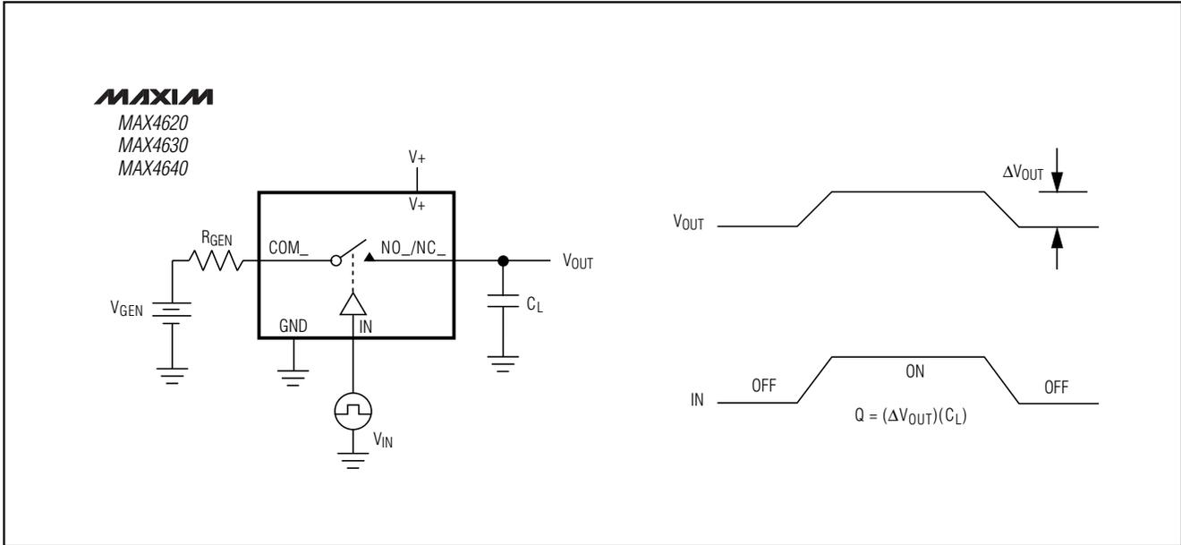
Figure 4. Charge Injection
