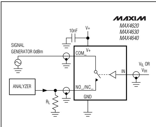
Figure 2. Off-Isolation/On-Channel Bandwidth
