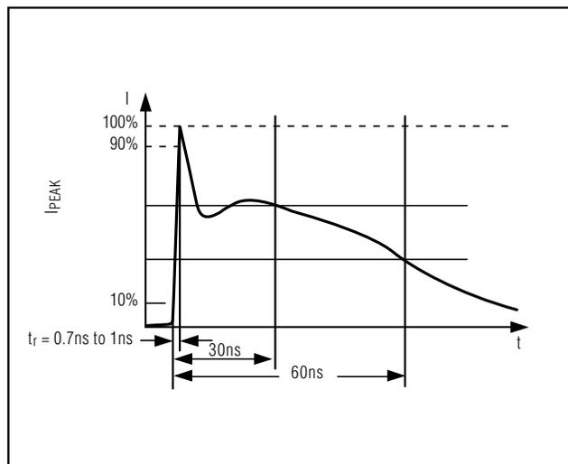
Figure 9. IEC 1000-4-2 ESD Generator Current Waveform
