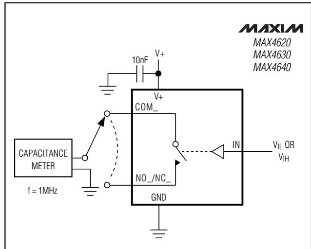
Figure 3. Channel Off/On-Capacitance
