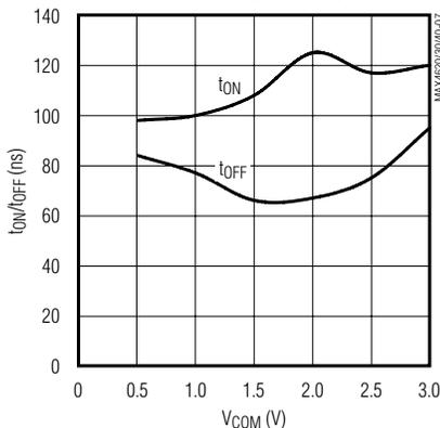
**TURN-ON/TURN-OFF TIME vs.  $V_{\text{COM}}$  ( $V_+ = +5\text{V}$ )**
