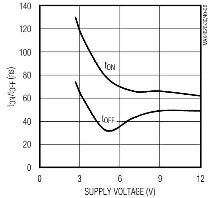
**TURN-ON/TURN-OFF TIME vs.  $V_{\text{COM}}$  ( $V_+ = +3\text{V}$ )**
