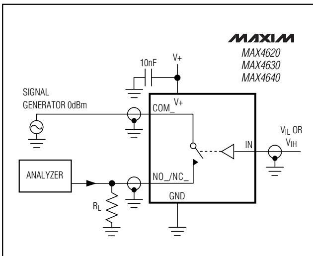
Figure 2. Off-Isolation/On-Channel Bandwidth
