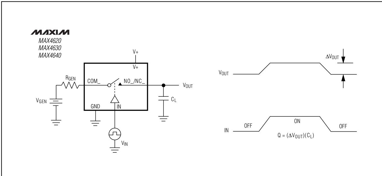
Figure 4. Charge Injection
