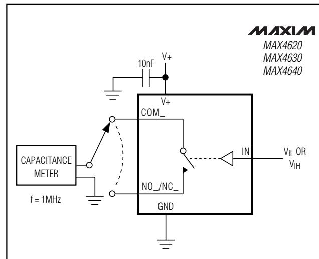
Figure 3. Channel Off/On-Capacitance
