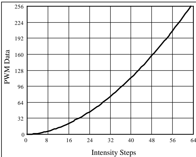
Figure 7 Gamma Correction (64 Steps)
