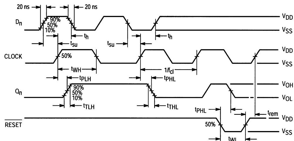
Figure 3. Timing Diagram
