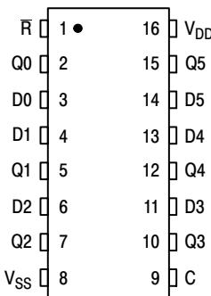
Figure 1. Pin Assignment
