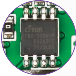
Figure 11-1: Flash memory module
