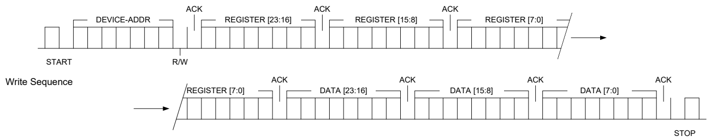
FIGURE 9. I 2 C WRITE SEQUENCE OPERATION
