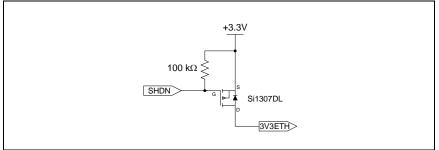
If using a circuit like this, be sure to power all ENCX24J600 VDD pins and the center tap of the Ethernet TX transformer through this power switch. It is invalid to disconnect VDD without removing power from the magnetics.
