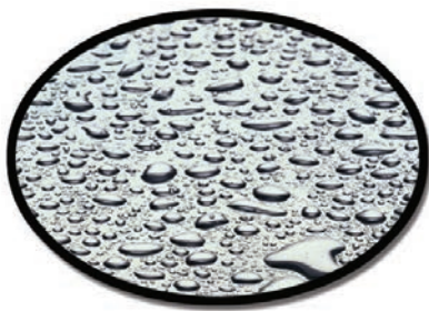
Solder beads off the porcelain coating like water on a freshly waxed car
