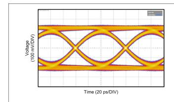
Figure 7. Typical Output Eye Diagram for the DS125DF410 Operating at 12.5 Gbps
