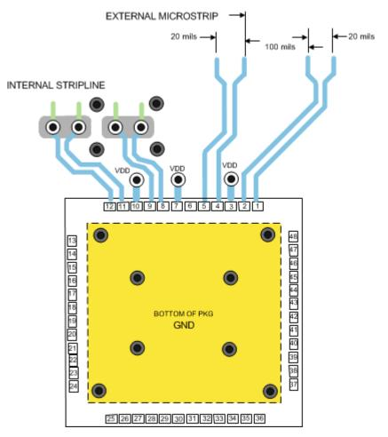
Figure 12. Different Transmission Line Topologies
