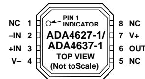
Figure 2. 8-Lead SOIC_N (R-8)
