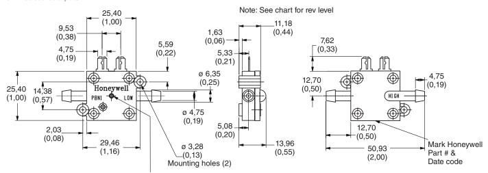
Adjustable Models Only Adjustment screw 1,27mm (,05) Hex socket - clockwise to increase actuation point, counterclockwise to decrease actuation point
