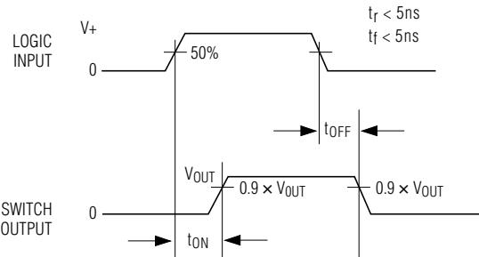
LOGIC INPUT WAVEFORMS INVERTED FOR SWITCHES THAT HAVE THE OPPOSITE LOGIC SENSE.
