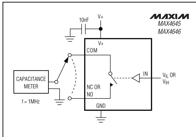
Figure 5. Channel Off/On-Capacitance
