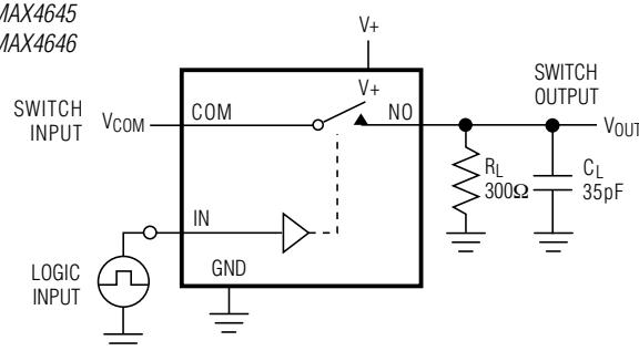
$C_L$  INCLUDES FIXTURE AND STRAY CAPACITANCE.
