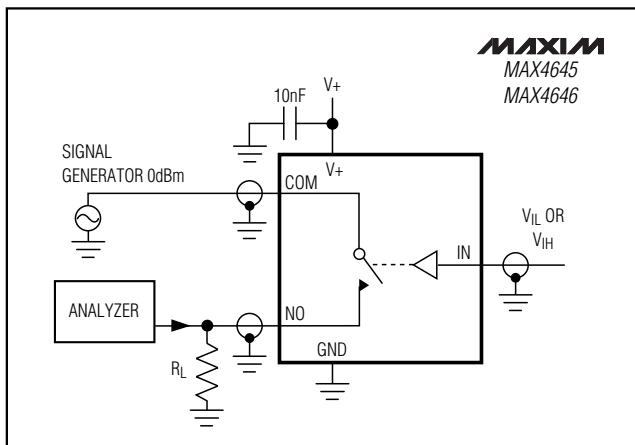
Figure 4. Off-Isolation/On-Channel Bandwidth
