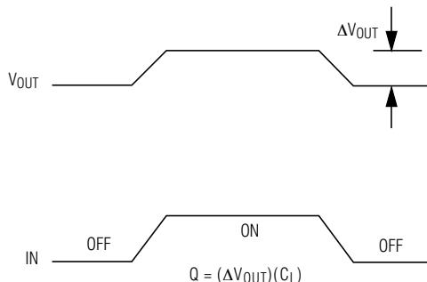
Figure 3. Charge Injection
