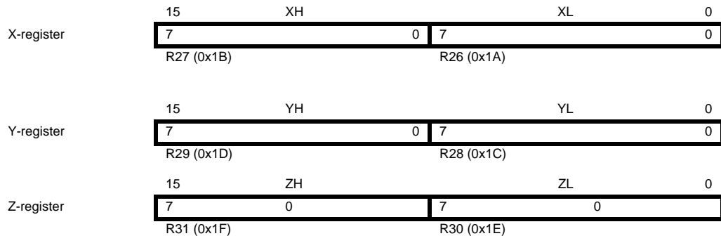
Figure 6-3. The X-, Y-, and Z-registers
