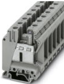
Feed-through terminal block, Connection method: Screw connection, Cross section: 0.75 mm 2 - 50 mm 2 , AWG: 18 - 1/0, Width: 15.1 mm, Color: blue, Mounting type: NS 35/7,5, NS 35/15, NS 32
