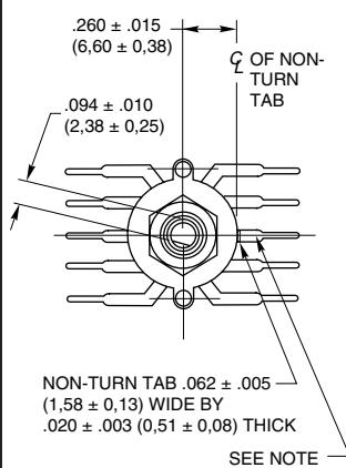
**Note:** Common location for a single pole per deck switch. For common location on multi-pole switches, see circuit diagrams.
