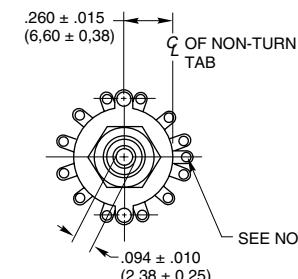
**Note:** Common location for a single pole per deck switch. For common location on multi-pole switches, see circuit diagrams.
