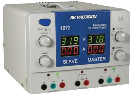
Model 1672, a Quad 3-Digit, Triple Output Regulated DC Power Supply has been added to B&K expanding new line of power supplies. Utilizing a standard 115VAC outlet as the power source, the new bench top unit provides the accuracy of quad 3-digit LED resolution, two variable voltage outputs of 0 to 32VDC/0 to 3A and one fixed 5VDC/3A output.
