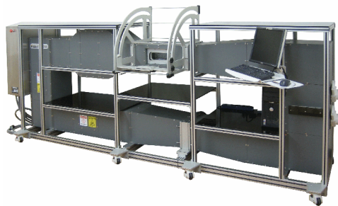
FDK Original Wind Tunnel
