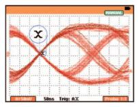
Dual-slope triggering used to capture the eye-pattern on a digital datastream.
