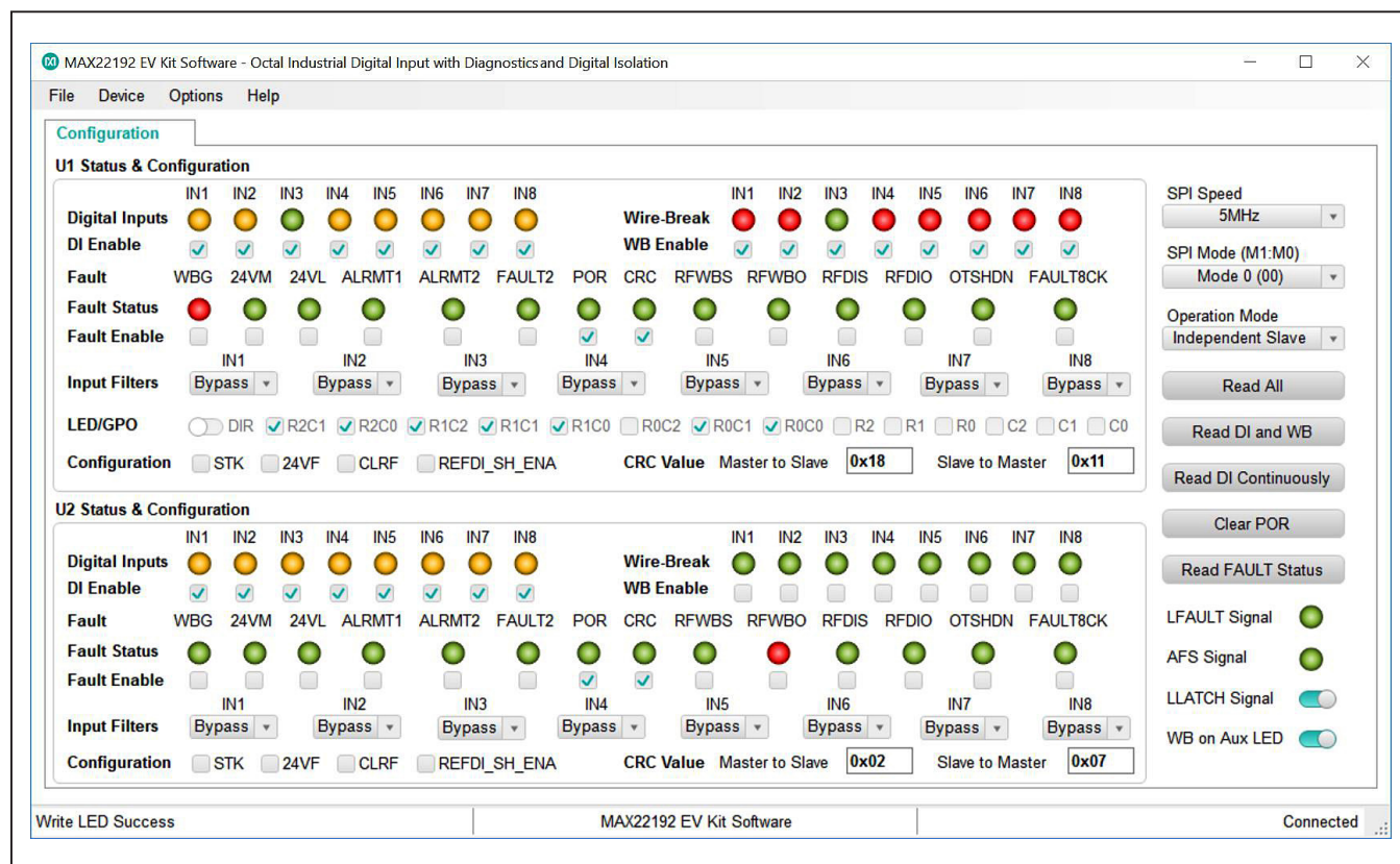
Figure 8. MAX22192 EV Kit Software—WB on Aux LED feature
