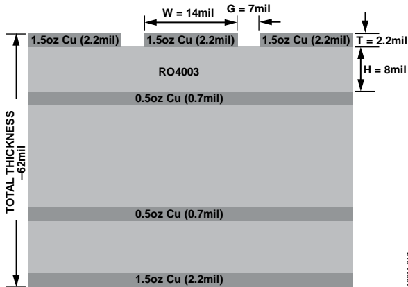
Figure 17. Evaluation Board (Cross Section View)
