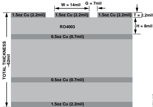
Figure 17. Evaluation Board (Cross Section View)
