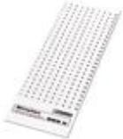
Marker cards, Card, white, Unlabeled, Can be labeled with: Plotter, Mounting type: Snap into tall marker groove, Snap into flat marker groove, For terminal block width: 6.2 mm, Lettering field: 6 x 6.1 mm
