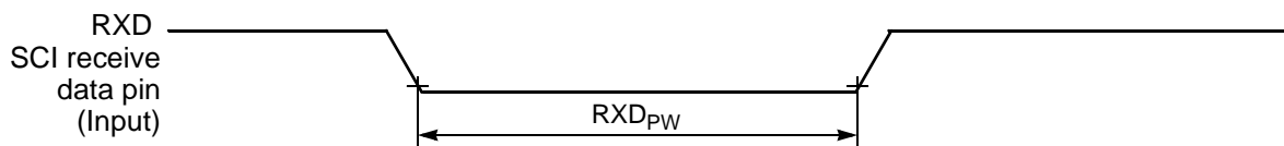
Figure 10-12 RXD Pulse Width
