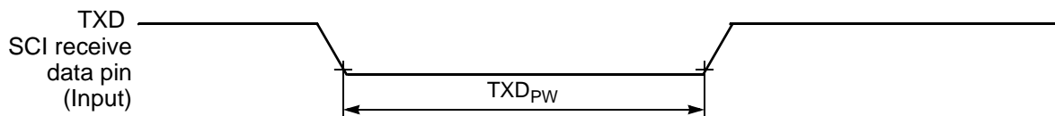
Figure 10-13 TXD Pulse Width
