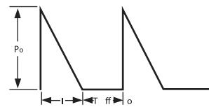
The Pulse Waveform, if other than square wave, must first be converted to an approximate square wave as shown below.
