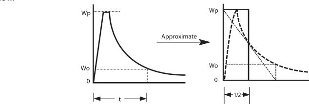
$W_p$  - Peak Power.  $W_o$  - Rated Power.  $t$  - Time to attenuate down to the rated power.
