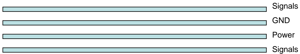
Figure 29: Typical 4-layer PCB construction
