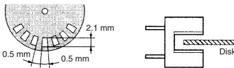
3. The following illustrations show the definition of response delay time. The value in the parentheses applies to the EE-SX498.
