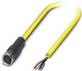
Sensor/Actuator cable, 4-position, PVC, Yellow RAL 1021, Free cable end, on Socket straight M8, Cable length: 5 m
