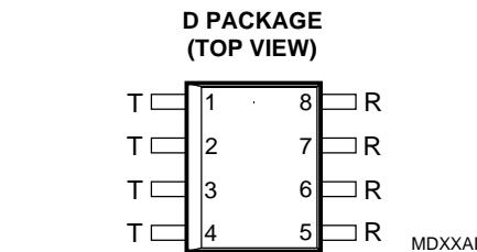
Specified ratings require the connection of pins 1, 2, 3 and 4 for the T terminal.
