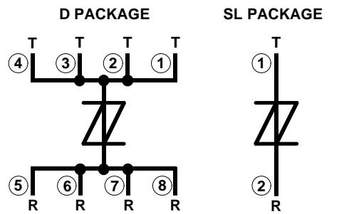
Terminals T and R correspond to the alternative line designators of A and B
