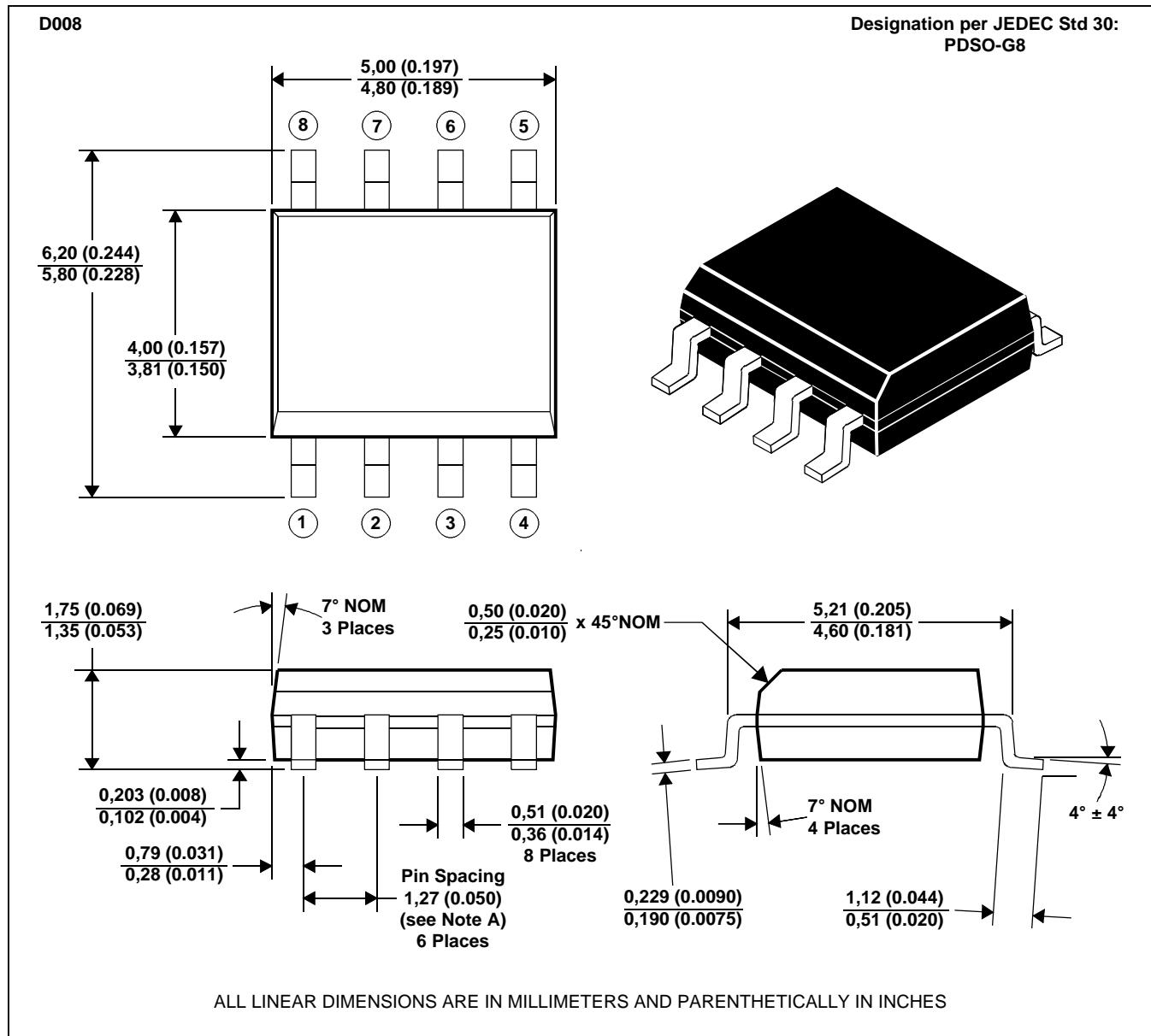
NOTES: A. Leads are within 0,25 (0.010) radius of true position at maximum material condition.
