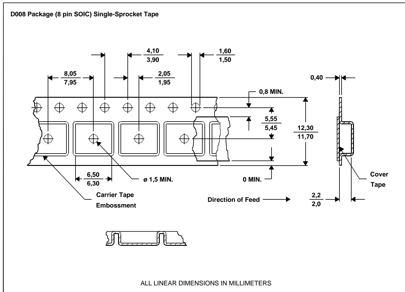
NOTES: A. Taped devices are supplied on a reel of the following dimensions:-
