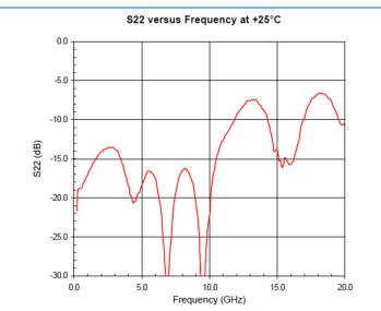
Note: The s-parameter gain results shown above include device performance as well as evaluation board and connector loss variations. The insertion losses of the evaluation board and connectors are as follows:
