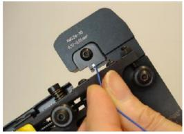
While keeping carefully the wire in position, close the handles until the ratchet releases.
