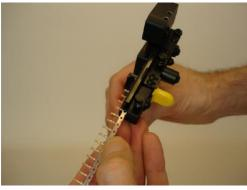
Once 50 mm of the contact strip is introduced into the terminal guide, the contacts can be fed one by one towards the crimp area. In order to do so, activate the manual feeder as shown on the pictures.
