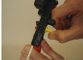
Feed a terminal into the crimping area of the hand tool.
