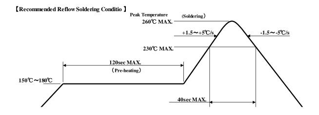
Notes 1 Temperature Profile for the reflow should be set to the surface temperature of resin which is on the top of LED. This should be the maximum temperature for soldering. Lowering the heating temperature and decreasing heating time is very effective in achieving higher reliability.
