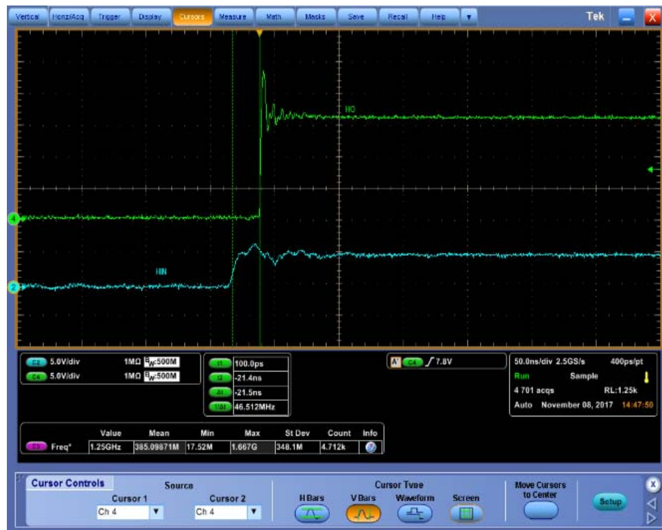
Figure 32. High Side Turn-Off Propagation Delay (NCP51530B)
