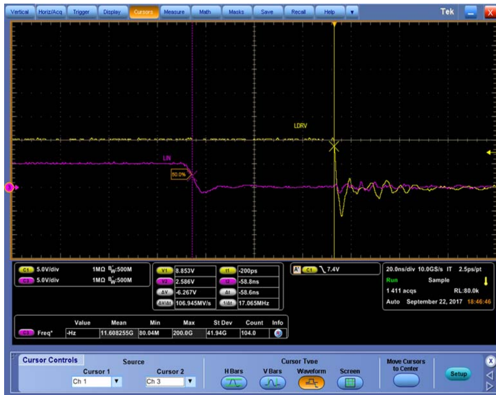
Figure 31. Low Side Turn-Off Propagation Delay (NCP51530A)
