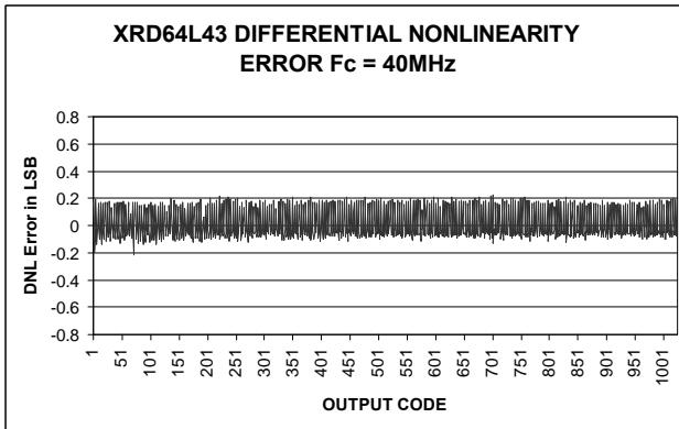
**Figure 8. Differential Non-Linearity, Differential Input Mode, Fc=40MHz, Fin=1.5kHz, VRHF=2.5V, V<sub>DD</sub>=3V**
