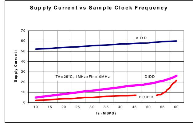
**Figure 17. Supply Current vs Sample Clock Frequency**
