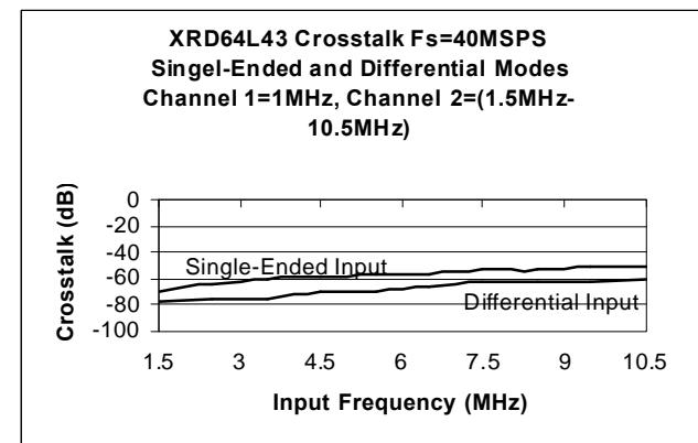
**Figure 11. Crosstalk vs Input Frequency, V<sub>DD</sub>=3V, Differential and Single Ended Inputs**
