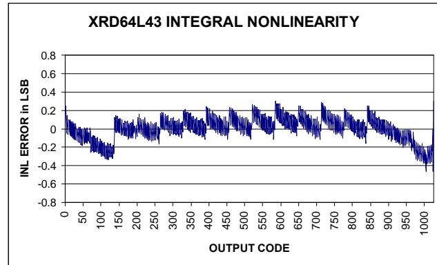
**Figure 9. Integral Non-Linearity, Differential Input Mode, Fc=40MHz, Fin=1.5kHz, VRHF=2.5V, V<sub>DD</sub>=3V**
