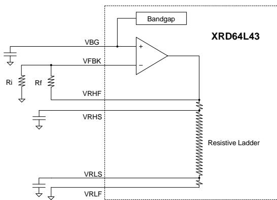
**Figure 2. Voltage Reference Generated from the Internal Bandgap Voltage w/gain**
