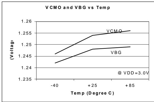
**Figure 18. VC MO and VBG vs Temperature**
