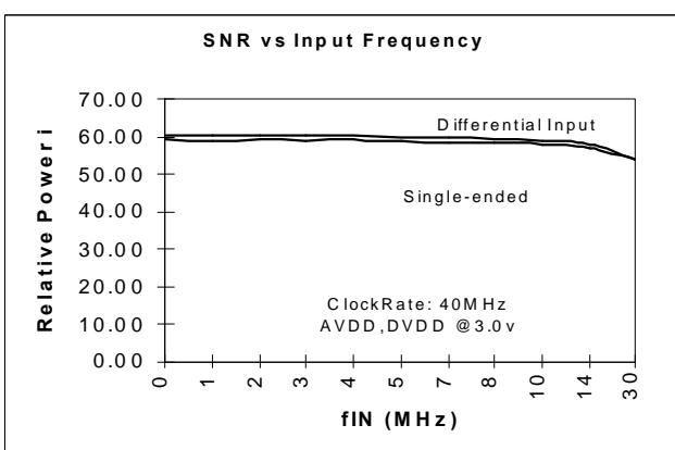
**Figure 15. SNR vs Input Frequency, Differential and Single Ended Inputs, V<sub>DD</sub>=3V**
