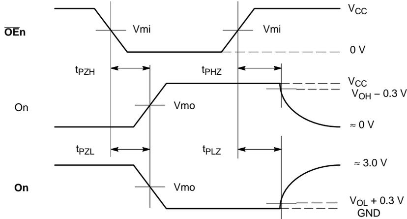
**WAVEFORM 2 – OUTPUT ENABLE AND DISABLE TIMES**
