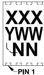
8-Lead 2x3 TDFN (MCP6H01, MCP6H02)
