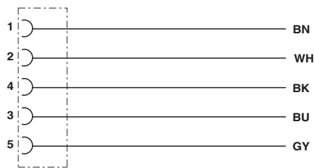
Contact assignment of the M12 socket
