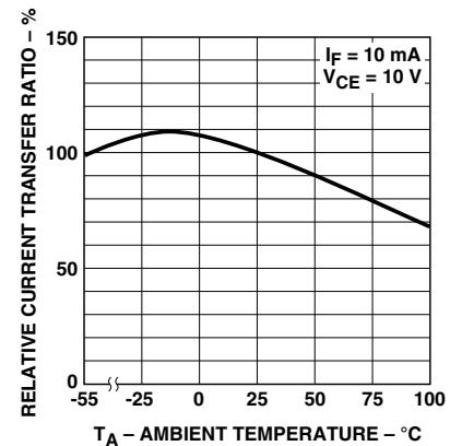
Figure 6. Relative current transfer ratio vs. temperature.
