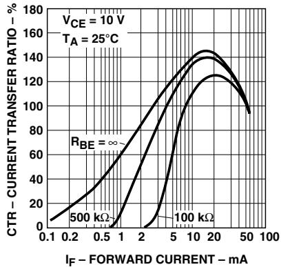
Figure 4. Current transfer ratio vs. forward current.
