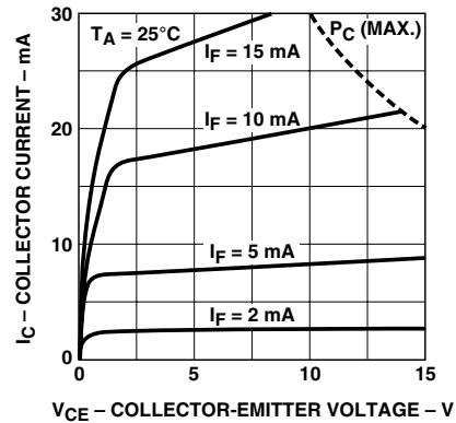
Figure 5. Collector current vs. collector-emitter voltage.
