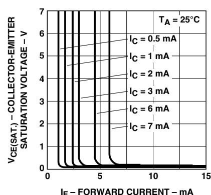
Figure 11. Collector-emitter saturation voltage vs. forward current.
