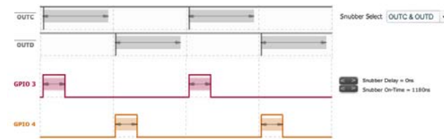
Figure 46. Active Clamp Snubber Configured on OUTx Signals
