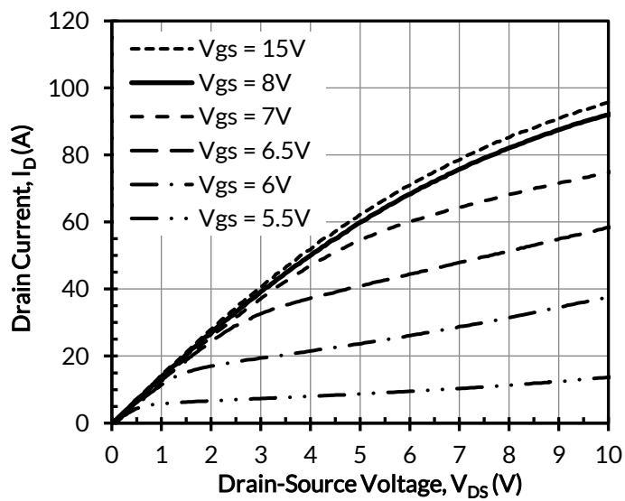
Figure 3. Typical output characteristics at  $T_J = 175^\circ\text{C}$ ,
