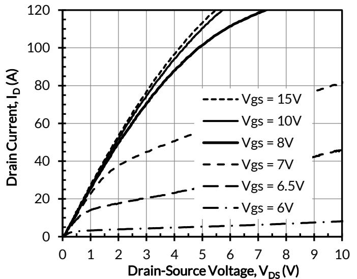
Figure 2. Typical output characteristics at  $T_J = 25^\circ\text{C}$ ,
