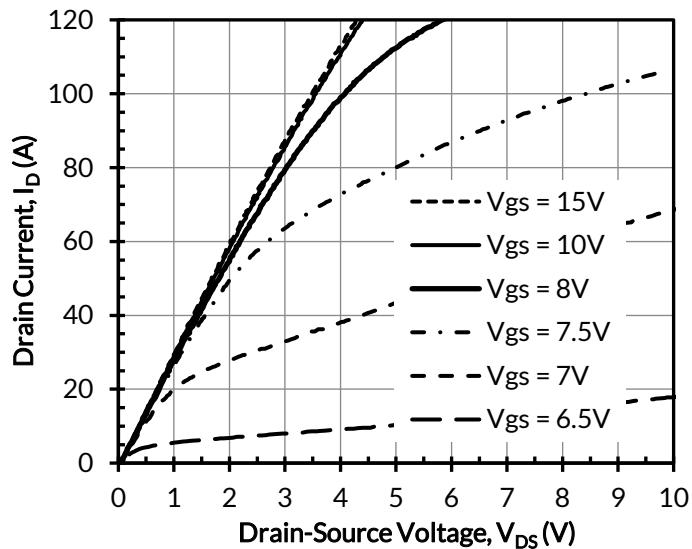
Figure 1. Typical output characteristics at  $T_J = -55^\circ\text{C}$ ,
