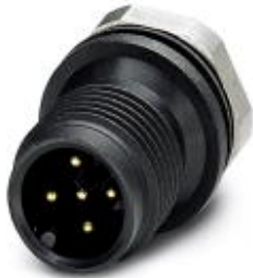
Sensor/actuator flush-type connector, male connector, 5-pos., M12, A-encoded, front/screw mounting with M12 thread, with solder cups, plastic version
