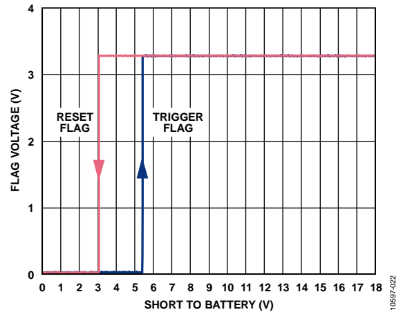
Figure 19. STB Output Response vs. Short-to-Battery Voltage on Outputs
