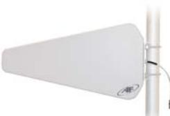
The Antenna Factor Log Periodic antenna is designed for long-distance directional communication over a wide range of frequencies. The DB1-LP antenna provides gain and directivity comparable to a Yagi, but in a much smaller overall form factor, and over a considerably wider range of frequencies. Constructed of UV stabilized materials, the antenna is suitable for long-term use in indoor or outdoor environments. The antenna includes complete mounting hardware for standard masts.
