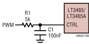
Figure 6. Dimming Control Using a Filtered PWM Signal
