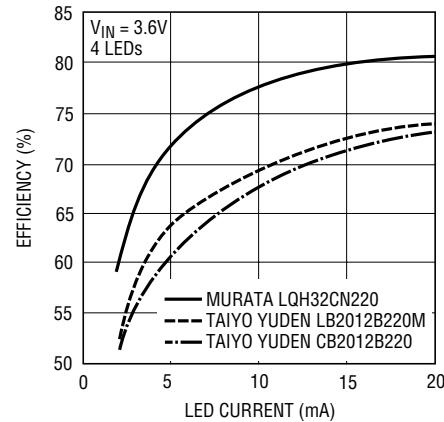
**Figure 4a. Efficiency Comparison of Different Inductors (LT3465)**
