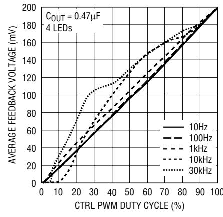
Figure 7d.  $V_{FB}$  vs CTRL PWM Duty Cycle
