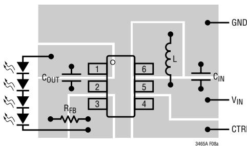
Figure 8. Recommended Component Placement.
