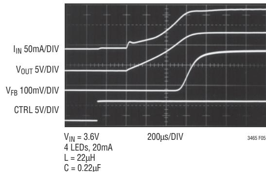
Figure 5. Start-Up Waveforms
