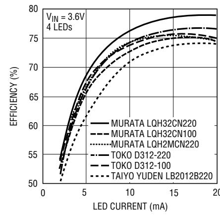
**Figure 4b. Efficiency Comparison of Different Inductors (LT3465A)**
