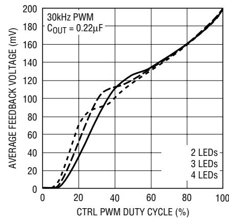
Figure 7f.  $V_{FB}$  vs CTRL PWM Duty Cycle
