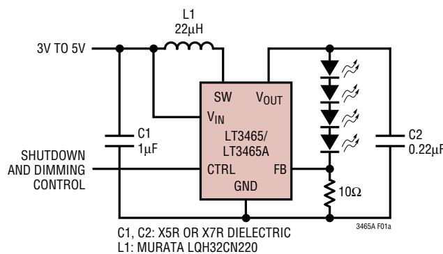
Figure 1. Li-Ion Powered Driver for Four White LEDs
