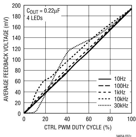
Figure 7c.  $V_{FB}$  vs CTRL PWM Duty Cycle
