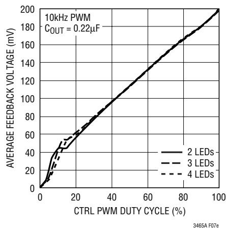
Figure 7e.  $V_{FB}$  vs CTRL PWM Duty Cycle
