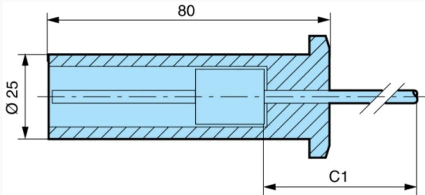
Protected electrode for mounting by suspension. Protective shell : PUC (S7) Electrode : stainless steel. Length of cable as requested (C1) : 79 696 001
