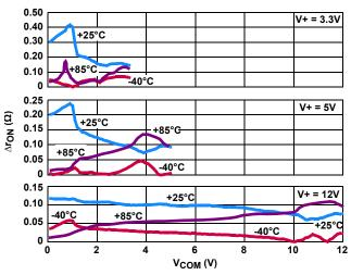
FIGURE 11. ron MATCH vs SWITCH VOLTAGE
