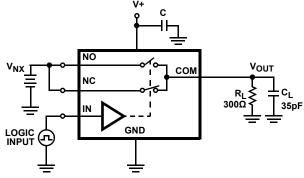
C<sub>L</sub> includes fixture and stray capacitance.
