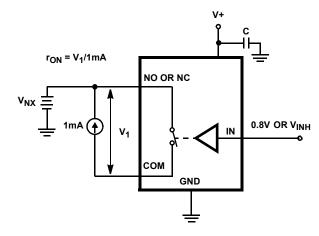
FIGURE 5. ron TEST CIRCUIT
