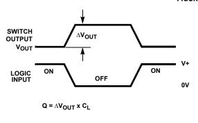
FIGURE 2A. MEASUREMENT POINTS
