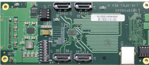
89KT0604S 2-lane, with I 2 C Configuration
