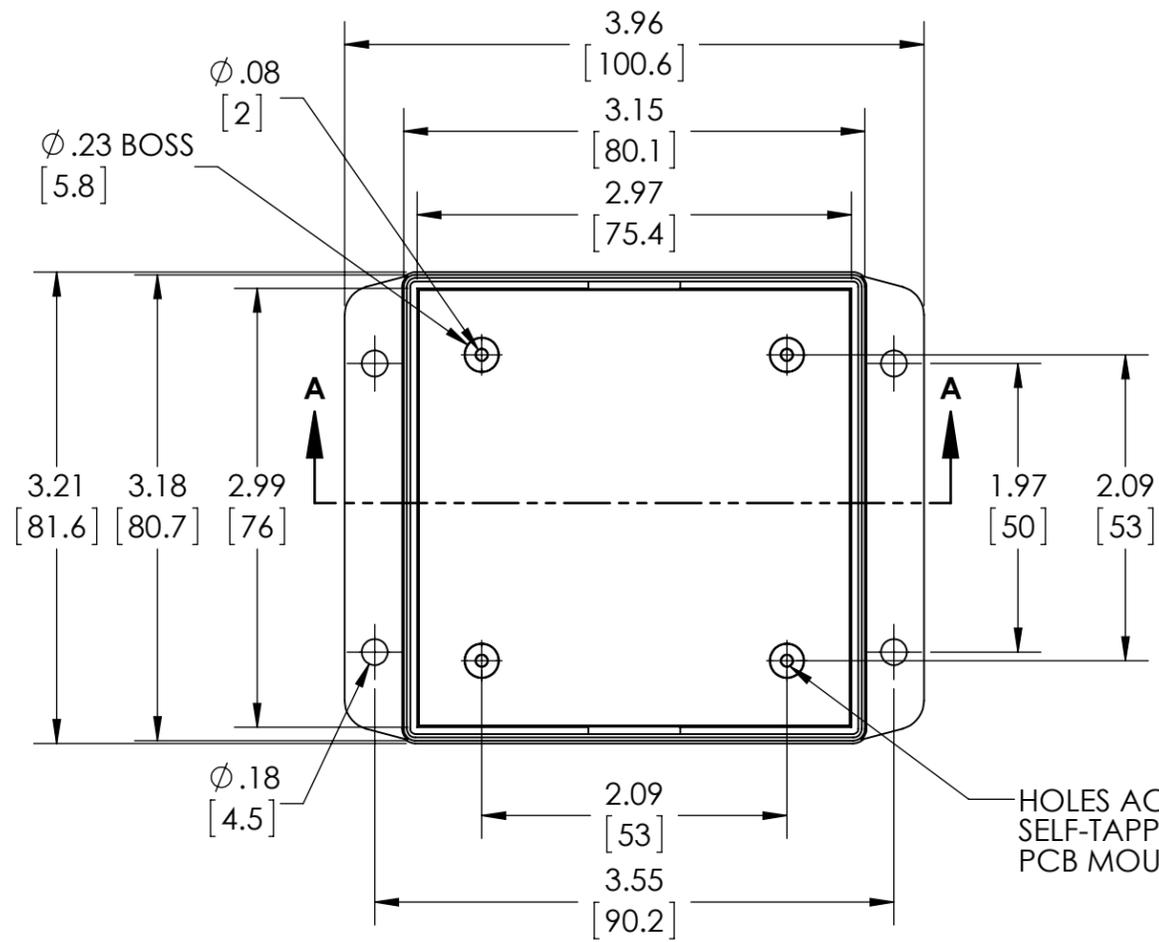
HOLES ACCEPT M2.6 x 6mm LG. SELF-TAPPING SCREWS FOR PCB MOUNTING
