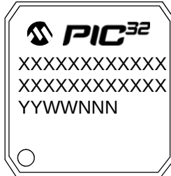
100-Lead TQFP (12x12x1 mm)
